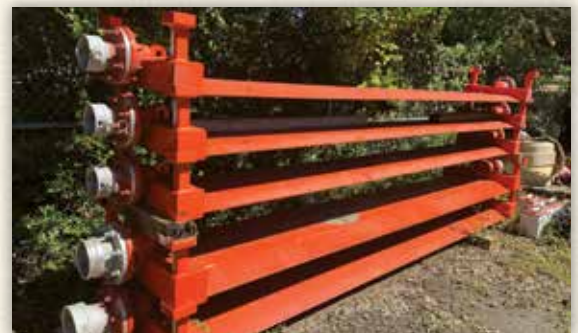
These road crossovers can be used to pump floodwater from one side of the road to the other. This eliminates the need to have hoses running across the road.
